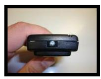
2. The probe case has two pieces that easily come apart once the screw is removed.
