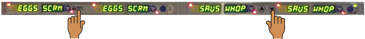
1. To change a bar address, disconnect the power to the unit. Reconnect power to the unit and immediately press and hold the **PC** button and **DOWN ARROW** buttons.
