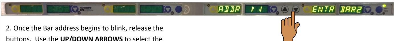
2. Once the Bar address begins to blink, release the buttons. Use the **UP/DOWN ARROWS** to select the desired bar address.
