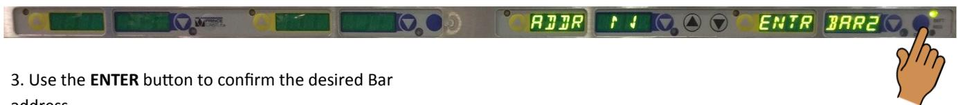
3. Use the **ENTER** button to confirm the desired Bar address.
