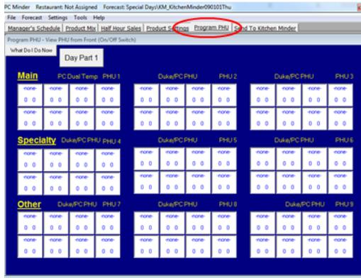
**2** Change *each* section to “PC Dual Temp” from “Duke/ PC PHU” by clicking on “Duke/ PC PHU” then selecting “PC Dual Temp”.
