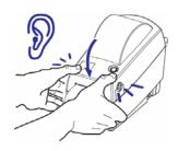
**4:** Close the printer. Gently swing the top cover down onto the printer's base. Press down on both sides until the cover snaps closed, typically with an audible sound.
