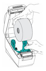
2: Open the label roll holders. Pull the labels guides open with your free hand and place the labels roll on the roll holders and release the guides. Orient the labels roll so that its printing surface will face up as it passes over the platen (drive) roller.
